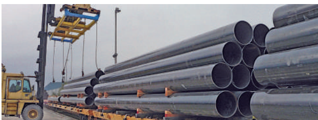
Bare steel line pipes are either sold to public utility companies or processed for coating
