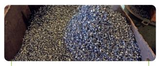
Steel scrap and alloys are imported/procured locally for melting and processing
