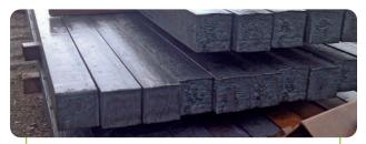
Billets are produced through a steel melting and ladle refining process. These billets are sold to rerolling mills or converted to rebars
