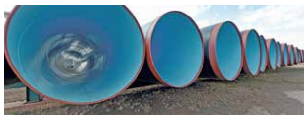
External and/or internal coating is applied to bare pipes
