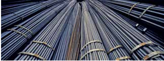
Re-rollers convert the billets into rebars and other long products.
