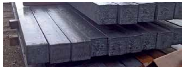
Billets are produced through a steel melting and ladle refining process. These billets are sold to re-rolling mills or converted to rebars
