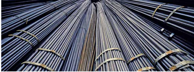
Re-rollers convert the billets into rebar and other long products.
