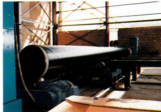
Three layer Polyethylene Coating being cut back at pipe ends for field jointing
